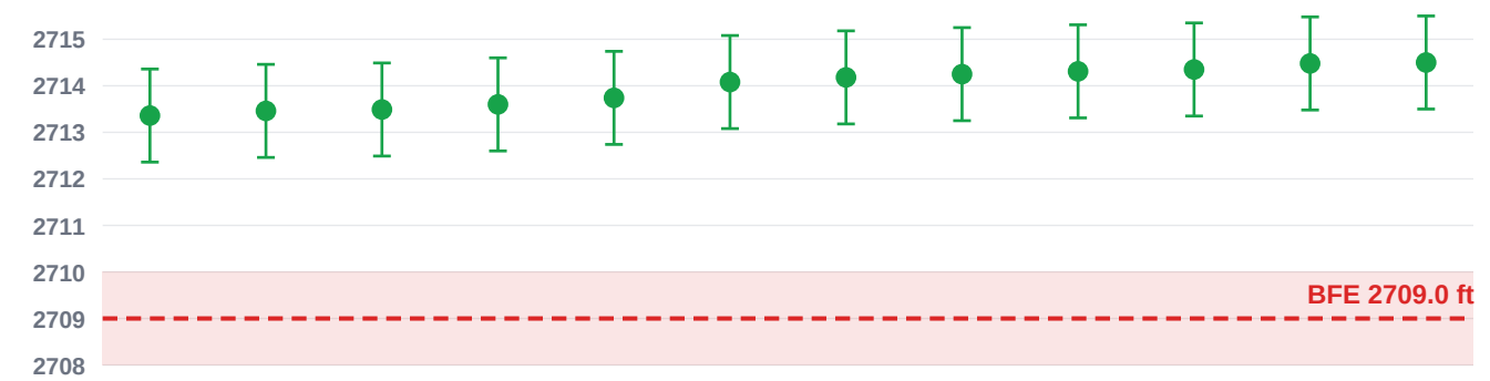
Sampled ground elevations (NAVD88 ft) ordered lowest to highest - the horizontal position is ordering only, not location. Whiskers show \pm 1.0 ft (95%) LiDAR vertical uncertainty for vegetated ground; the shaded band around the BFE line shows its rounding and interpolation uncertainty. Green = at/above BFE, red = below. See the plan view below for where each sample sits.
